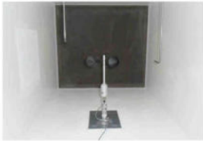
Photo of the Anemometer in the Wind Tunnel
